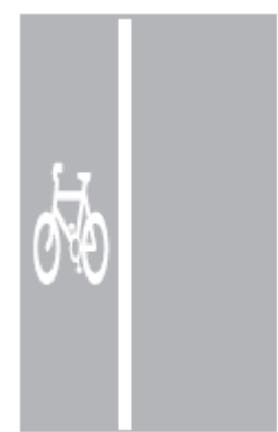
Road markings for a mandatory pedal cycle lane
