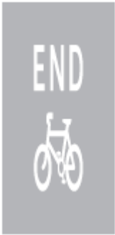
Road marking indicating the end of a cycle lane, track or route
