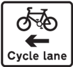
Pedal cycle lane on road at junction ahead or (where "lane" is varied to "track") cycle track crossing road at junction ahead
