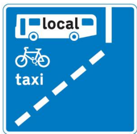
With-flow bus lane ahead which pedal cycle and taxis may also use
