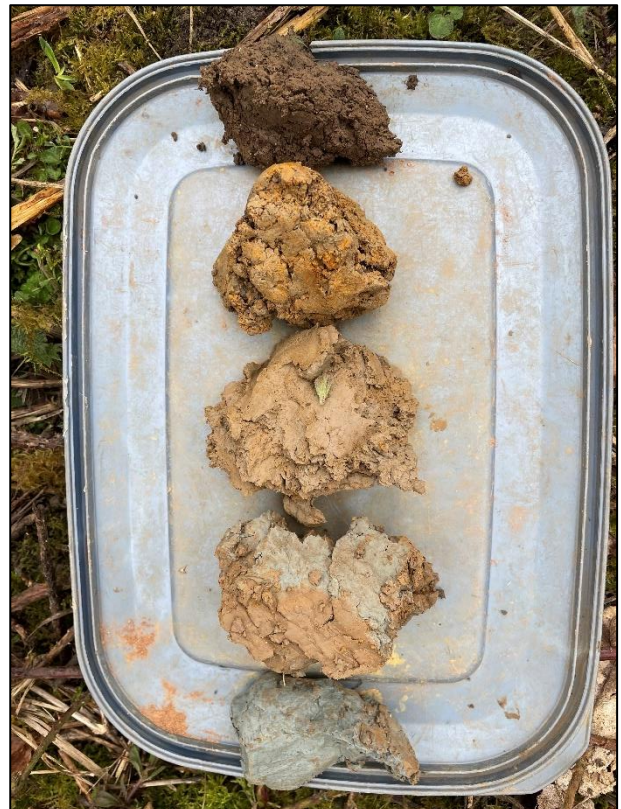
Figure 22. Soil samples from 0.1 m to 4.09 m – TP1.
