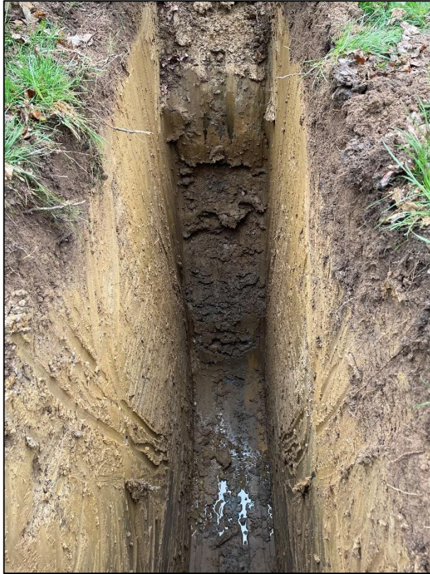
Figure 25. CLAY topsoil over CLAY subsoil – TP3. Note minor seepage in base.
