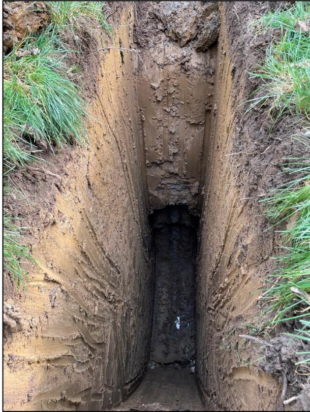
Figure 27. CLAY LOAM topsoil over CLAY subsoil – TP4. Note minor seepage in base.
