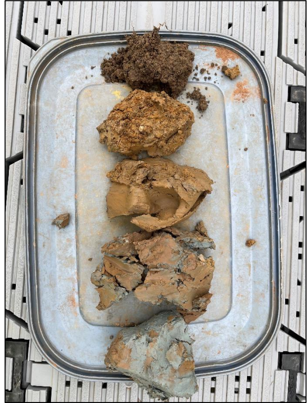
Figure 26. Soil samples from 0.1 m to 4.0 m – TP3.
