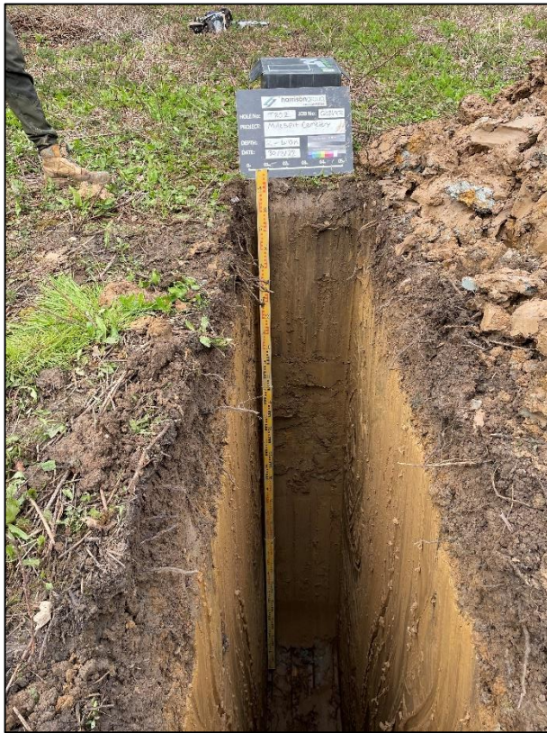
Figure 23. CLAY topsoil over CLAY subsoil – TP2.
