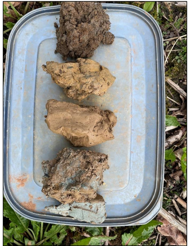
Figure 24. Soil samples from 0.1 m to 4.0 m – TP2.
