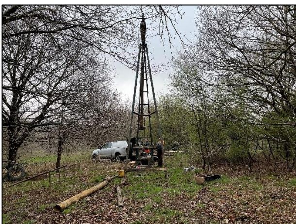
Figure 31. Dando 2000 Cable Percussive Rig.
