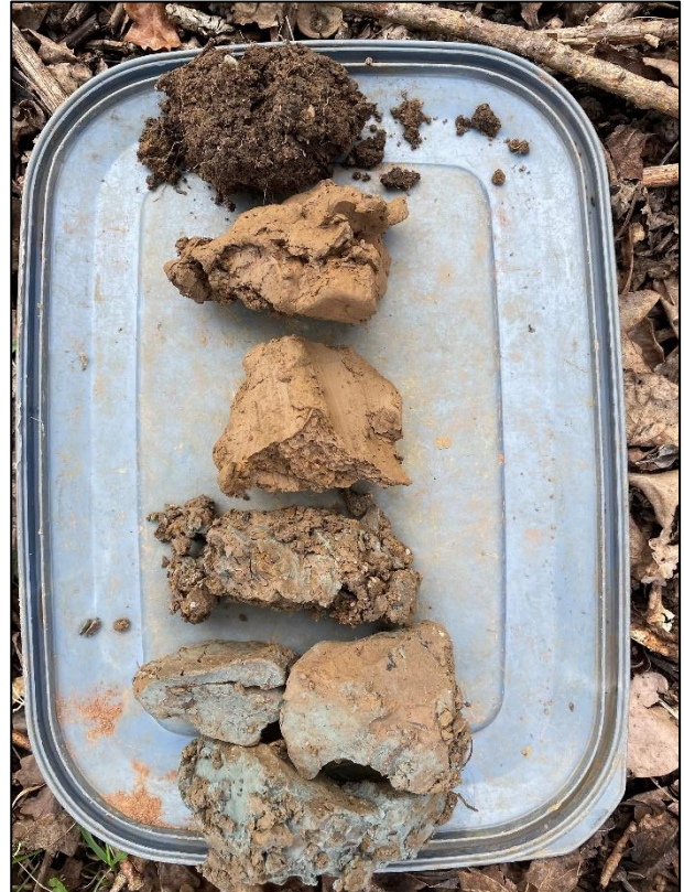
Figure 30. Soil samples from 0.1 m to 4.0 m – TP5.
