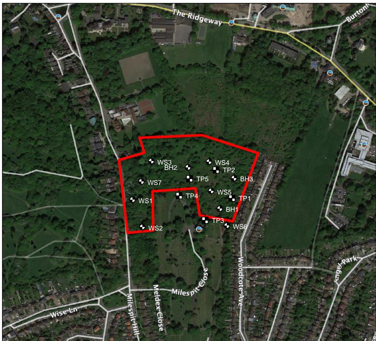
Figure 1. Site location (within the red line – courtesy of Peter Mitchell Associates). TP1 to TP5 mark the approximate locations of the test pits observed during the site investigation. BH1 to BH3 and WS1 to WS7 mark the approximate locations of cable percussive boreholes and dynamic continuous sampling boreholes (courtesy of Harrison Group Environmental Ltd).
