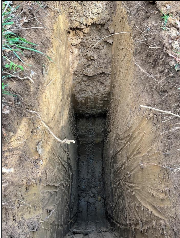
Figure 29. CLAY LOAM topsoil over CLAY subsoil – TP5.
