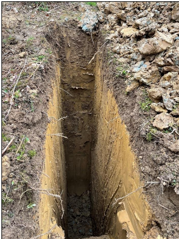
Figure 21. SILTY CLAY LOAM topsoil over CLAY subsoil – TP1
