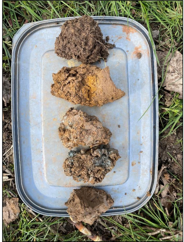
Figure 28. Soil samples from 0.1 m to 4.0 m – TP4.
